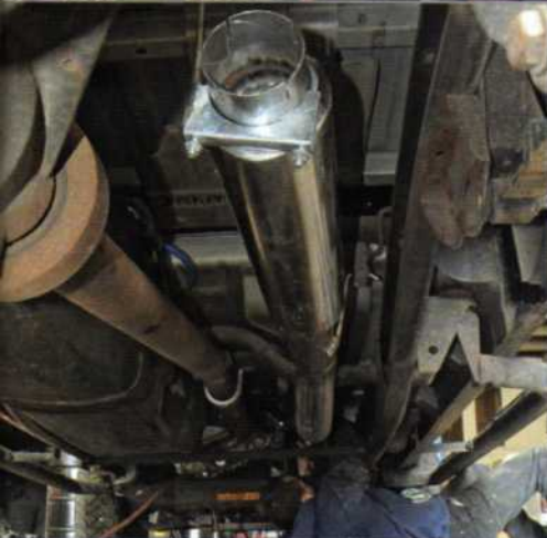
(top left) Mandrel bends mean that the tubing is not welded or crushed. It maintains its 4-inch round diameter from one end to the other. (top right) The core of the Silverline muffler. (lower left) High quality clamps and hangers made the install a piece of cake. (lower right) Black Max is coming along quickly in the appearance department, with Iron Bull bumpers front and rear, 20-inch Mamba M3 wheels and a Trailmaster lift. Stay tuned for more upgrades (and repairs) to this project.
